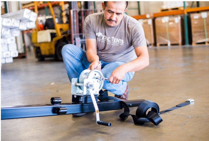
STEP 3: Uncoil the Canopy Jack Strap and attach the looped end to the bolt on the web winch. Again you will need a wrench and socket to tighten. Advance the winch to load the strap onto the winch spool. Leave enough slack to allow the webbing to pass to the top and back down to the bottom of the jack.
