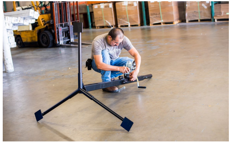
STEP 2: Attach the winch mechanism to the Canopy Jack Lite Base using the following: 3 each 3/8" x 1" Hex Bolt, 6 each 3/8" Washer, 3 each 3/8" Locking Hex Nut. To tighten this connection you will need a wrench and socket (Size 9/16").
