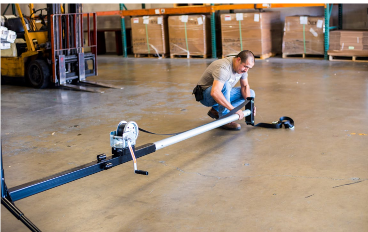
STEP 5: Install the aluminum mast to the top of the base and connect the top roller to the top of the mast. These connections lock into place with a side release push button. Assure as you assemble that the webbing continues to stay straight without twists.
