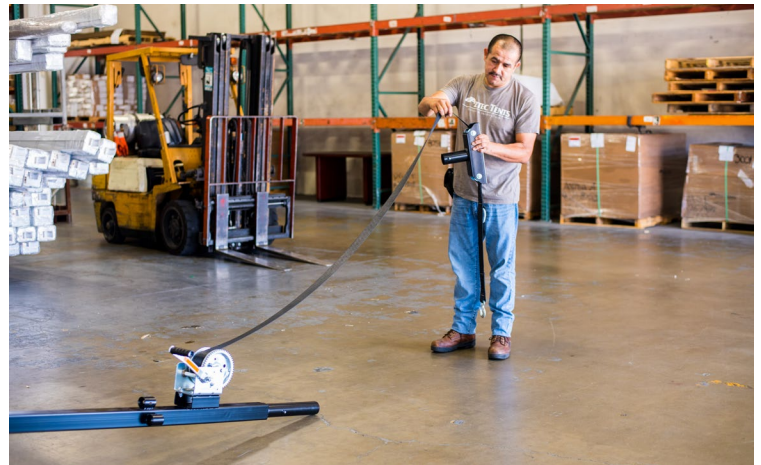
STEP 4: Pass the hook end of the Canopy Jack Strap through the Canopy Jack Lite Top Roller. The webbing should sit on top of the two silver rollers then pass back out the other side. Make sure there are no twists in the webbing leaving the winch to the top roller.
